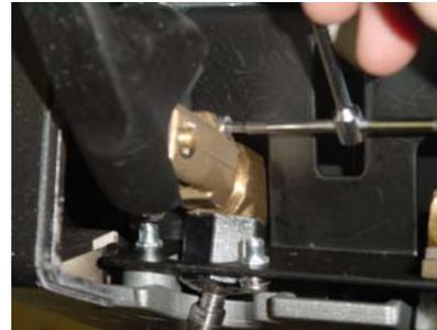
To remove the lever and fork, release the set screw using 3 mm allen wrench. When the screw is released you will be able to remove the fork and lever together, as show in picture 2. **Note when replacing the fork and lever system make sure there is no play in the lever.**
