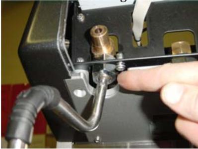
This picture shows the lever section of the swivel wand. This section of the wand can become worn. To remove, unthread the nut from the valve. When removed, replace the lower oring in the bottom of the nut and upper oring on valve body. **Beware there is a spring and a bushing that will come out with the wand.**
