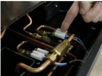
This inspection checks the flowmeters for any corrosion that may have built up on the terminals. Please make sure there is no water, coffee or foreign substance. This could cause a short circuit.
