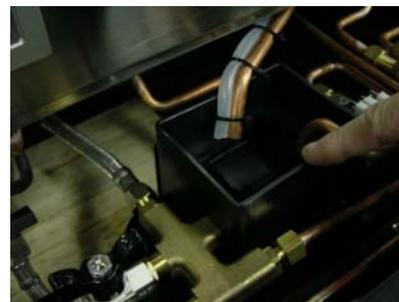
The drainage system needs to be checked often by the owner and when service is scheduled. The drain could or will be clogged with coffee or other foreign material.
