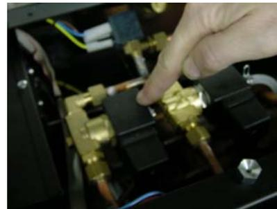
Many of the Nuova products use a hot water dispenser. In some models we use a hot and cold water mixing system. If a failure of any valve occurs, you will have water leaking out the hot water wand continually. Replacement of the valve may solve the problem.
