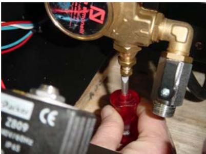
Pump adjustment clockwise will increase pressure, counterclockwise will decrease pressure. All adjustments for this pump are underneath the machine. Be sure to unlock the locking nut before making the adjustment.
