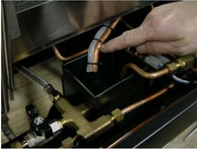
In this picture, watch the discharge tube for leakage when you are back flushing the brew head. If water comes out during the brew cycle there is a problem with the group valve. Possible replacement will be necessary. Aggressive back flushing with detergent may resolve the problem as well.
