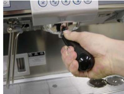
On this check you are checking the Alignment of the portafilter. The portafilter should not exceed 15 Degrees past center. If this occurs one of 3 options will solve your problem: replace the group gasket, add shims or replace the portafilter.
