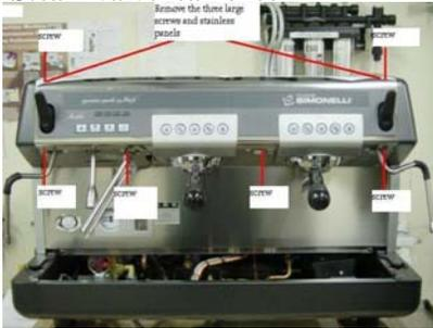
When the espresso machine has reached a certain age or usage, parts start to fail. Those parts are usually orings. Each steam valve has a set of orings. When there is a problem typically the problem will show itself. The steam wand will leak continually when the lever is in the off position. This would require service. This booklet will show you how to access the Aurelia front panel to service the steam valve.
