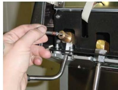
This picture is showing the removal of the piston rod. The piston rod has two orings. These should be replaced and lubricated every 6 months.
