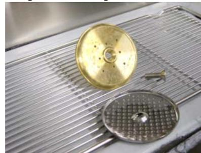
This inspection checks the dispersion plate for any coffee or liquid build up. Which could cause uneven distribution of water over the fresh ground coffee. If caked with coffee, please demonstrate hot to backflush the machine and recommend doing this once a day.
