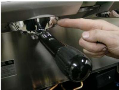
During the back flush procedure, if you see dripping down around the group ring. It may be possible your group valve is leaking. Replacement of Two orings will correct the problem.
