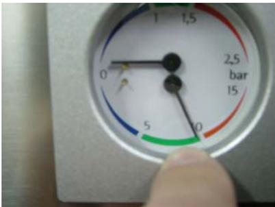
When you switch the brew switch on, you will see the pump pressure increase to 9 bar. This pressure is standard pressure when brewing espresso. The diagram below shows the pump adjustment.
