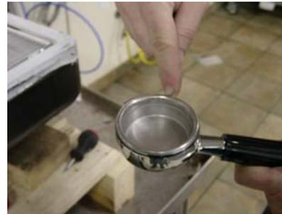
This inspection shows the person if there are any dents, dings or cracks in the basket Also look for dirty baskets. This check also needs to inspect the handle for cracks.
