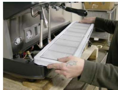
For this inspection, please remove the drain tray. Once the drain tray is removed look for the drain box. Also engage the portafilter with the blind filter. Press the continuous pro button and look for water seeping of the coffee tubing in drain cup.
