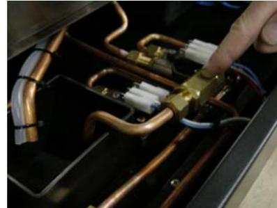
This test is going to tell you if the expansion valve is leaking. To perform the test you must back-flush the group and watch the valve for any leaking. If it leaks during this cycle replacement is necessary.
