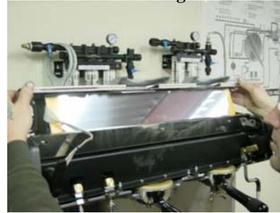
When the housing has been reversed this will allow you to gain access to the steam valves. Pay careful attention to the ribbon cable.
