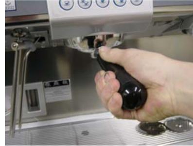
This procedure allows the machine to be worked with extreme pressures. During this time its important to inspect all parts of the machine for leaking.
