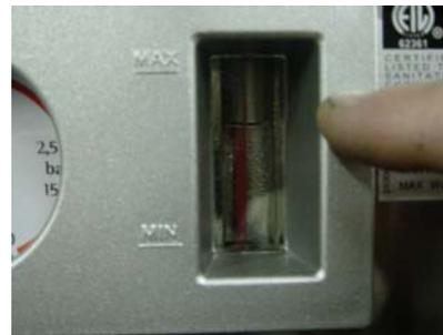
Most all Traditional espresso machines use a level glass to show the water level in the tank. It is important to take note of the water level during servicing of the machine. Water level will range from 1/2 to 3/4 full.
