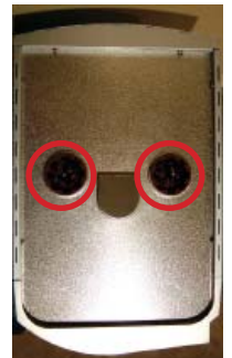
TOP VIEW OF MACHINE WITH GRINDER COLLARS CIRCLED
