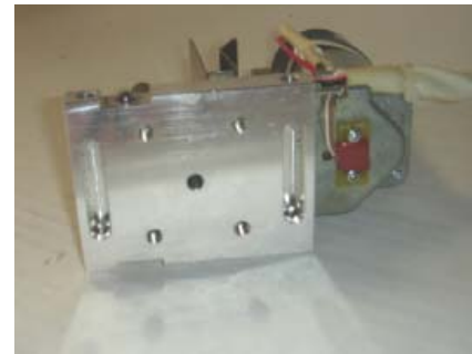
View of the Bottom of the Mounting Plate: you can access the gear box through the hole in the bottom of the mounting plate. This way you can manually control the piston.
