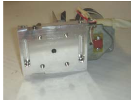
VIEW OF THE BOTTOM OF THE MOUNTING PLATE: you can access the gear box through the hole in the bottom of the mounting plate. This way you can manually control the piston.
