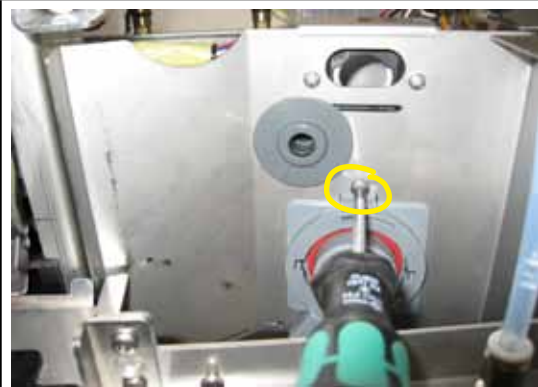
fig. 8: dismantle mixer motor
